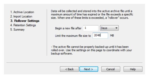
This page configures the conditions that trigger creation of a new datastore file. Datastore files are "rolled over" based on a time or size policy (whichever is reached first). Files may be configured to roll over after a fixed amount of time (from one hour to 365 days) or after reaching a maximum size (100 MB to 2 GB).
