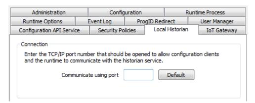
**Communicate using port:** This parameter specifies the TCP/IP port that the server Runtime and Configuration use to communicate with the Historian Service. The valid range is 1024 to 65535. The default is configured by the server.
