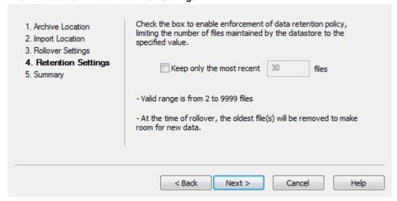
This page is used to optionally specify the maximum number of datastore files Historian retains. When a rollover causes the file count to exceed this value, the oldest datastore file is deleted. The valid range is 2 to 9999 files.
