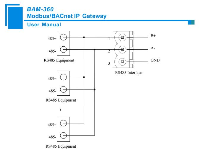
When RS485 communicates under the point-to-multipoint mode, in order to prevent the reflection and interference of the signal, it requires connecting a terminal resistor in the farthest two ends of the each line; the parameter is  $120\Omega \ 1/2W$ . There are no parallel terminal resistors at the serial port side of BAM-360.
